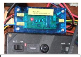
Fig. 2. Compass-radar (NMEA) interface in *Ragged Robin*.
